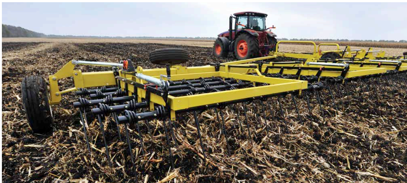
Figure 3.3. Tine harrow implement for mechanical control of weeds in pulse crops.
